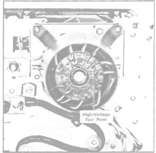
Fig. 6-5. Location of high-voltage test point (rear panel, protective cover removed).
